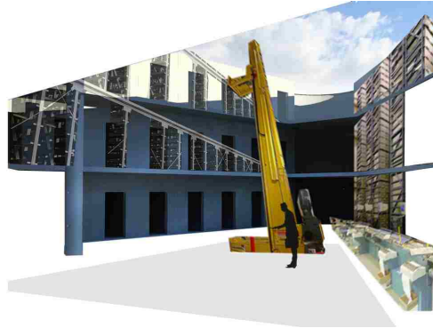
Figure 25 Automated storage integrated into the existing prison cell blocks.
